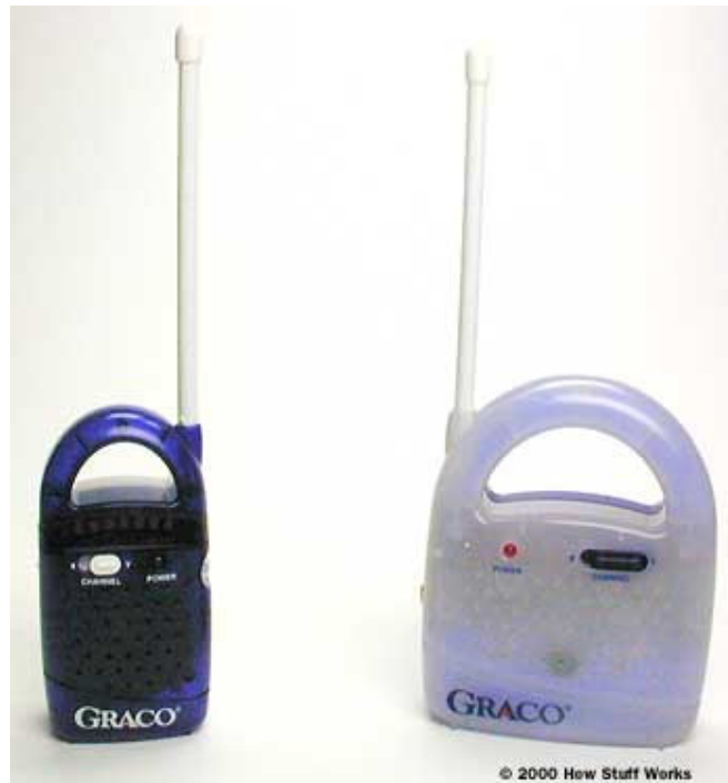
A typical baby monitor, with the receiver on the left and the transmitter on the right: The transmitter sits in the baby's room and is essentially a mini "radio station." The parents carry the receiver around the house to listen to the baby. Typical transmission distance is limited to about 200 feet (61 m).
