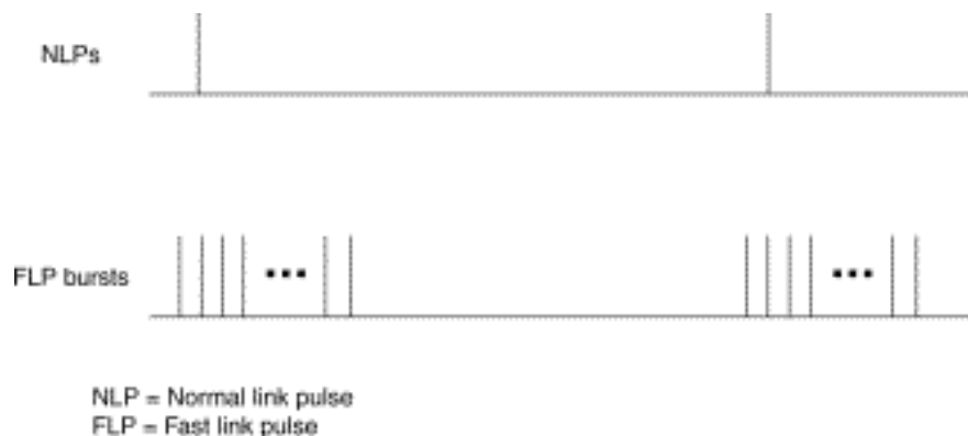
Figure 7-27: Autonegotiation FLP Bursts Replace NLPs During Link Initiation
